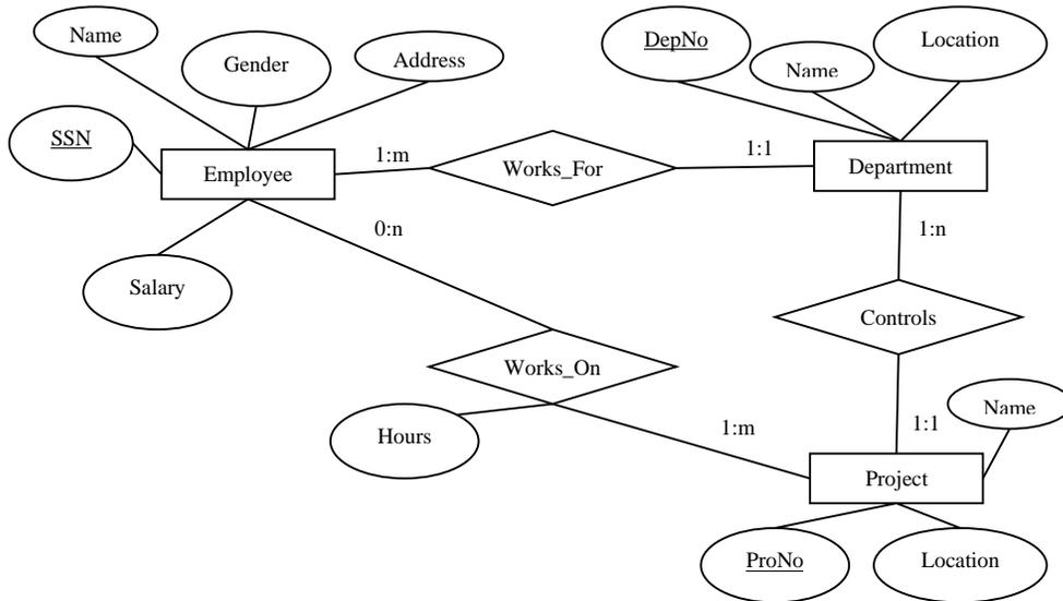
Figure 3 Example of an ER Diagram S
